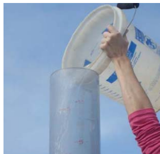
Figure 9: Filling Infiltrometer With Water
